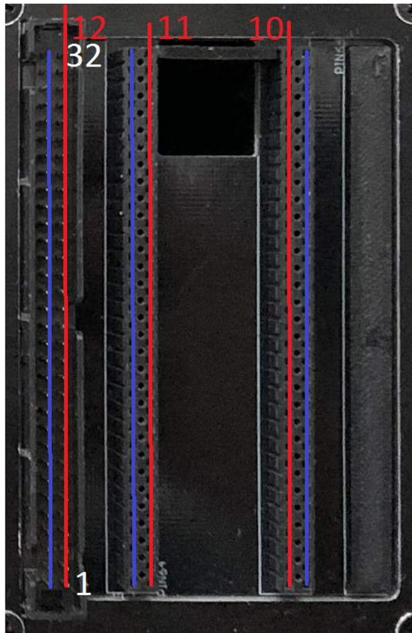
Figure 3: The pin layout of IDC sockets.
